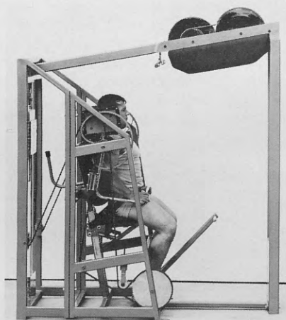
Over 240 degrees of rotary resistance is provided in the primary movement in a Nautilus Pullover/Torso-Arm Machine.
